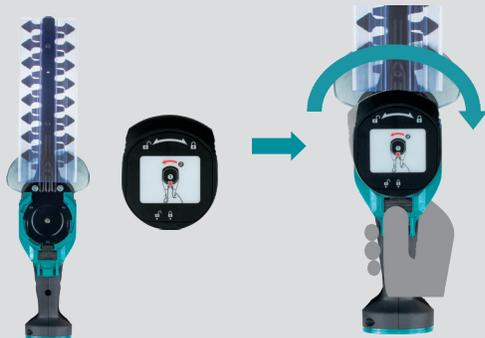
Place the undercover by lining the □ with the ▲ on the tool. Confirm that the lock lever is in the groove of the undercover. Then, while pressing the undercover in, turn the undercover clockwise until the □ aligns with the ▲ on the tool.
